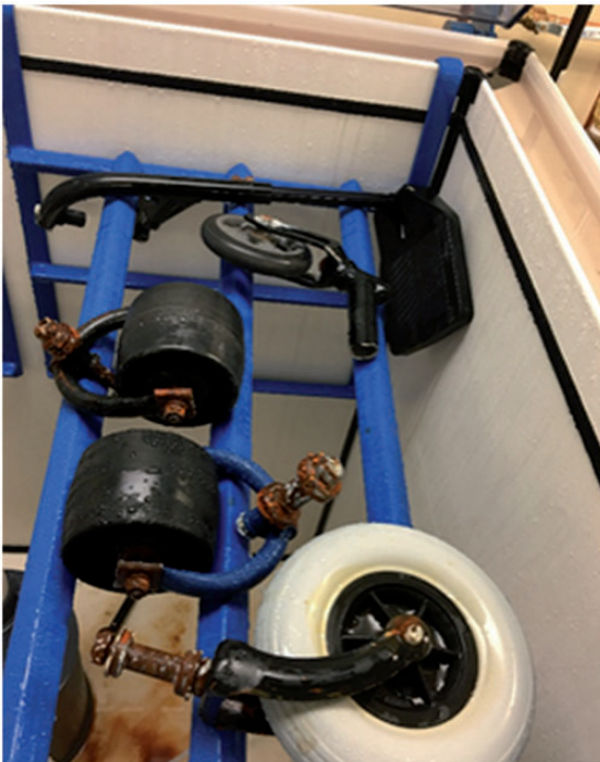
Figure 4. Salt fog test equipment for corrosion exposure. 21
